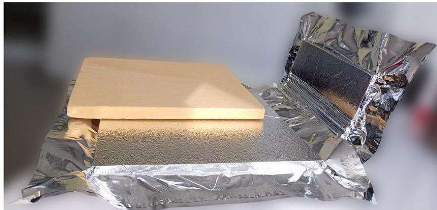
The Cannon Afros LIFE VICORPAN project aims to demonstrate how to enhance the energy efficiency and recyclability of Vacuum improved Insulation by **CORe** shaped **PANe**ls of commercial and domestic refrigerators. Photo: Cannon Group.
